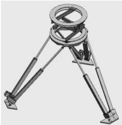
Fig. 2 Simplified Stewart Platform Mechanical Drawing
