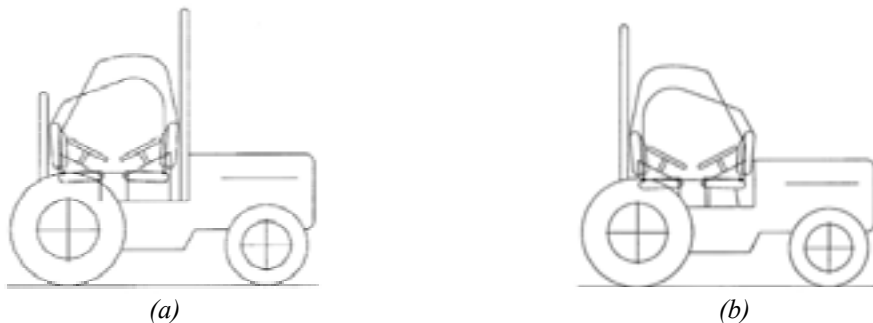
Slika 2: Mogućnosti ugradnje zaštitnih ramova na upotrebljivanim traktorima ispred rukovaoca, (b) iza rukovaoca Fig.2: Possibilities of installing protective frames on used tractors (a) in front of the operator, (b) behind the operator
